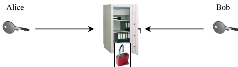
Fig. 6.2 Analogy for symmetric encryption: a safe with one lock
